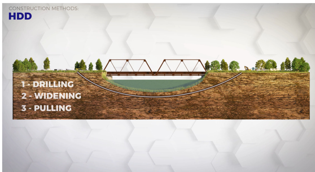
Figure 7-9: Horizontal Directional Drilling Approach
